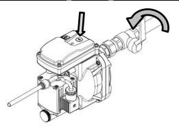
Remove Ø8 tube from push connection.
