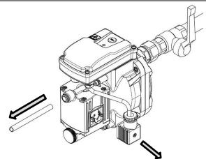
Unscrew four screws and carefully remove complete valve assembly by pulling it aside like shown.
