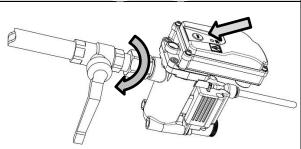
Remove strainer insert and clean it. At the same time, check integrity of mesh.
