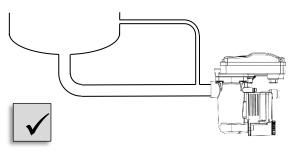
If if the bottom connection is used, the height of the upper connection must be lower than the lowest point of the condensate level. Upper unused connection must be properly sealed
