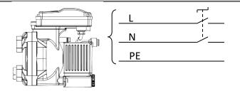
Do not connect EMD after protection device of heavy inductive load like compressor motor (left). Instead, heavy inductive load and EMD should be protected separately (right).
