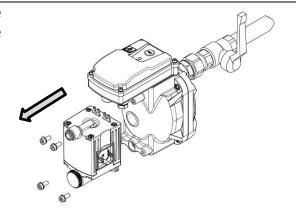
Install new valve assembly. Make sure that the O-ring and connector gasket are positioned correctly.
