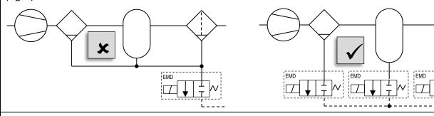
Drainage piping must be built without traps that would trap air in the EMD and prevent condensed water to enter it (left). Additional venting would not help because debris collects in the lowest part of drainge pipe and clogg it (right).
