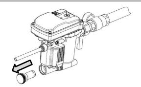
Clean also O-ring sealing and its gland thoroughly. Otherwise, strainer sealing may start to leak.
